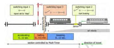
2. The locomotive stops in front of the signal until the hold time has expired (and switching input 1 has been switched to "open" automatically) or until switching input 1 has been opened (e.g. by means of an external switch).
