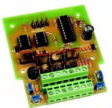
Time switch for analogue and digital model railway layouts
