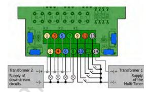
Choose operation mode 1 (r) for testing all outputs, so do not insert a jumper to any of the solder pins ( $\rightarrow$  section 8). Set a short switching time (trim-pot as far as it will go to the left). Then check all four outputs and switching inputs one after the other.
