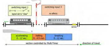
**Example 2: Signal set to "Clear"** (switching input 1 open)
